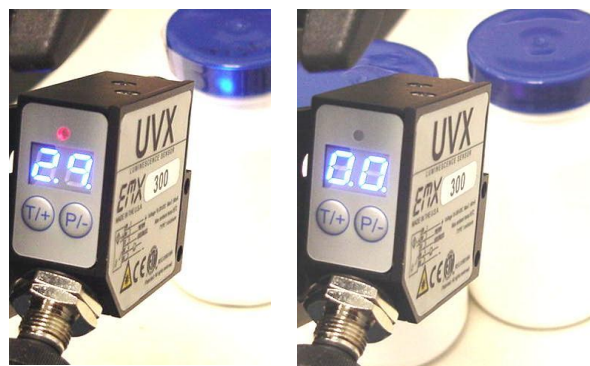
Tamper seal present Tamper seal missing
