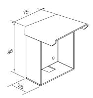
Metal box for wall mounting of model P41. Epossidic painted. Colour grey. Material: zinc-coated iron.
