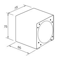
Metal box for wall mounting of model P40. Epossidic painted. Colour grey. Material: zinc-coated iron.
