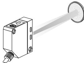
This system is limited by the fact that shining or reflecting objects cannot be identified by the sensor as they reflect the emitted light, as if they were reflectors.
