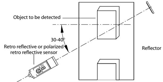
**N. B.:** The adjustment obtained in point 7 is the most efficient for shiny and/or semi-transparent objects; if the objects to be detected are opaque and non-reflecting, the trimmer can be brought to the extreme clockwise position which will allow the photoelectric sensor to operate even in very dusty environments.
