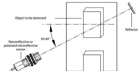
N. B.: The reflex and polarized reflex photoelectric sensors should never be used for maximum range values in the presence of adverse environmental conditions (such as dust, smoke, etc.) which could reduce the efficiency of the sensors.
