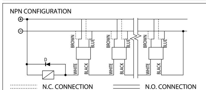
NOTE: In presence of inductive loads, when more sensors are connected in series, diode D should be connected in antiparallel to the load.
