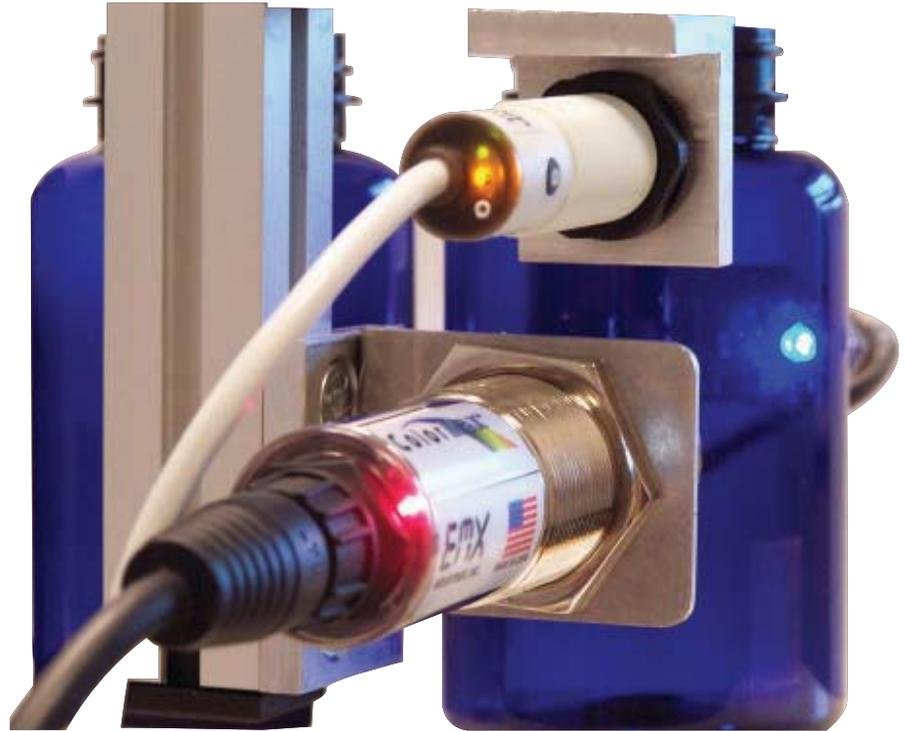
Optical sensors are fast becoming indispensable in manufacturing for the power, time and cost savings they offer. Here, a color sensor verifies the color of a plastic bottle in a manufacturing setting. Courtesy of EMX Industries Inc.
