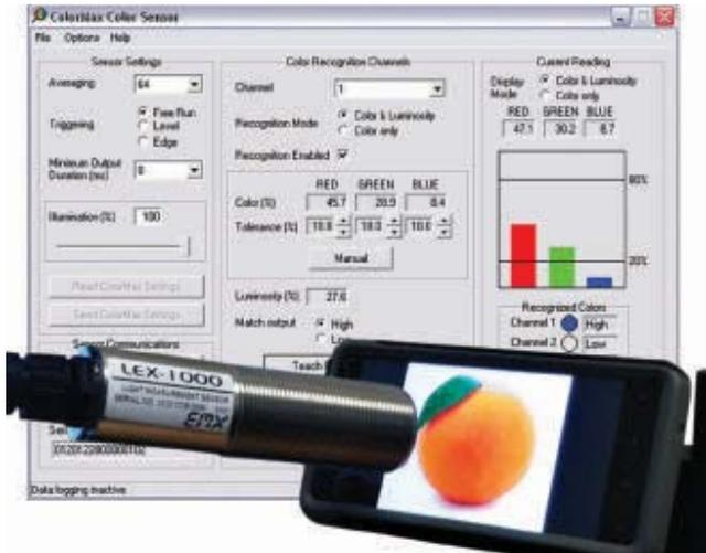
This light-analysis sensor is analyzing the RGB values of a display for an industrial application. Courtesy of EMX Industries Inc.
