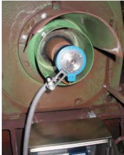
A fiber optic encoder keeps watch in a steel rolling mill in Germany. Courtesy of Micronor Inc.
