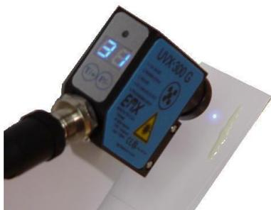
The photo on the left shows the sensor set at 30mm from a 92 bright paper envelope. The 2-digit display shows a relative intensity signal level from 0 through 99. The 92 bright paper reads 31. The indicator above the display shows the status of the discrete output, currently off.
