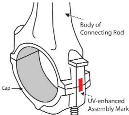
Figure 1. An assembly mark in UV-enhanced ink guides workers in installing connecting rod caps correctly, and can be read down the line by a UV fluorescence sensor for QC purposes.
